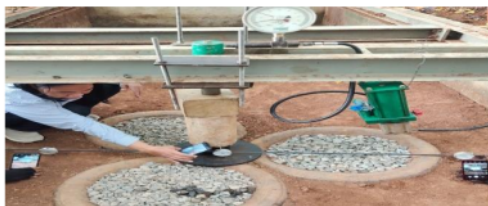
Fig 14 : Horizontally arranged tire foundation model test
